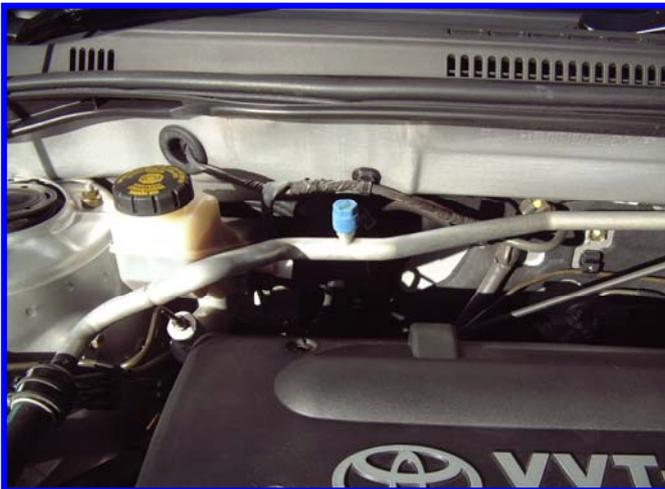
2. The small blue cap in the close-up on the left, covers the low-pressure port of the car air-con's gas system. It's here that top-up gas is added
